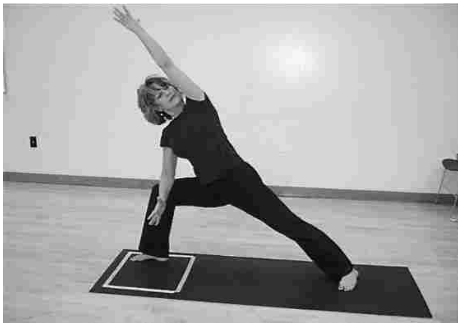
Figure 1.—Condition 1. Force plate perimeter is outlined on yoga mat and subject begins sequence by standing over the force plate. Forces are measured in either one or both lower and upper extremities.
